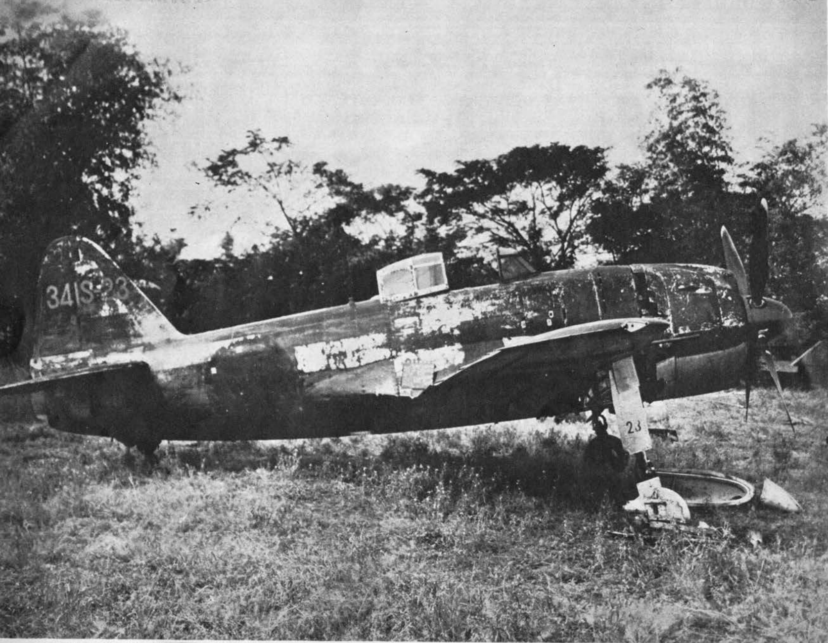
GEORGE Newest and best protected of Japs' single-engine fighters, George has a top speed of over 400 m.p.h. Thick fuselage and mid-wing set it off from other Japanese fighters.
